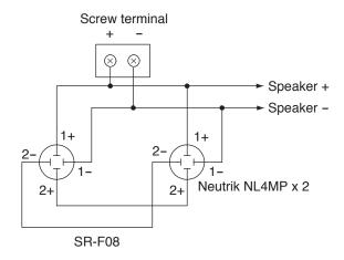
Two speakers can be parallel-driven in a cascade configuration as shown at right.
